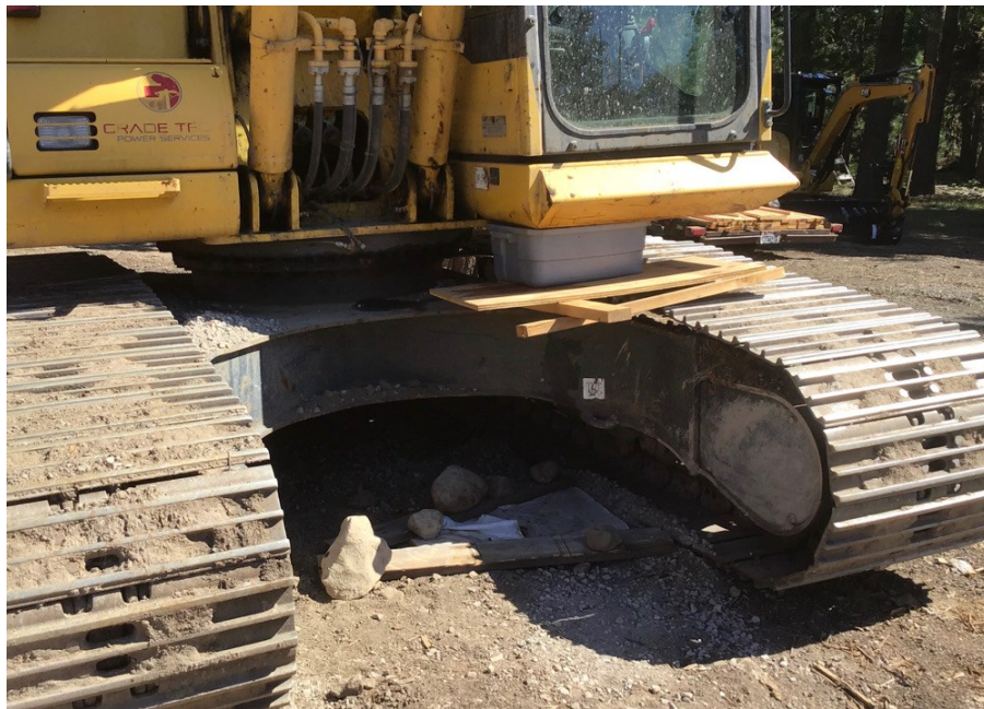
Photo 6: Excavator with leakage being adequately contained with tubs/pans in accordance with APM HAZ-2
